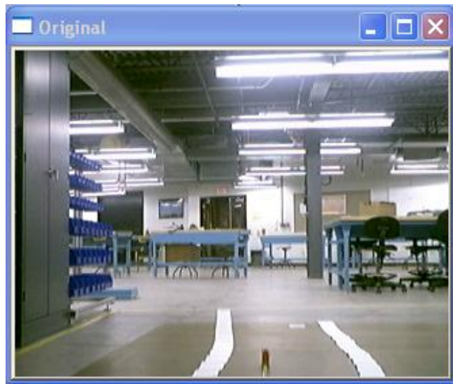
Figure 10: Camera captures image. White tape was used to simulate boundary lines.
