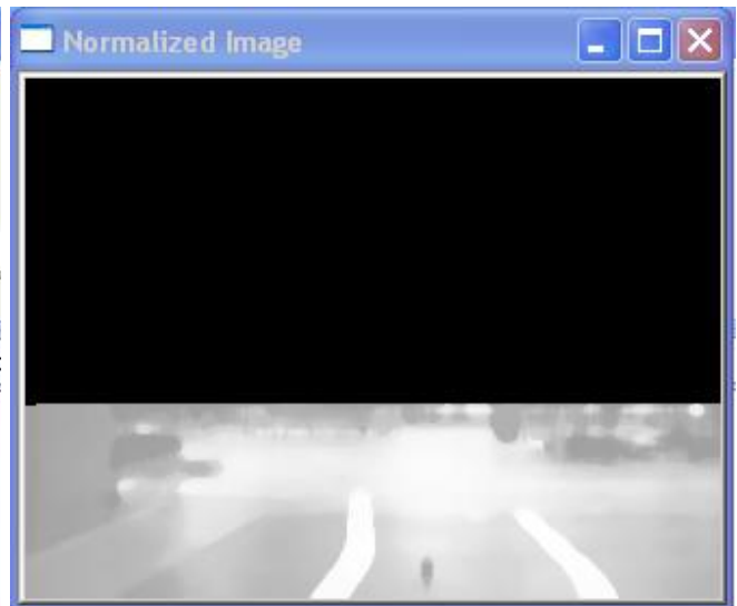
Figure 11: The image is gray scaled, and top half of the image is ignored to minimize false detections. The image is smoothed using OpenCv function cvSmooth() . This function looks at each pixel's neighboring pixel intensity to determine its actual intensity. This eliminates the random white pixel in the grass, and makes the boundary lines a more consistent intensity.
